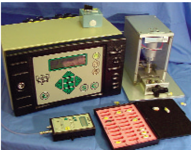
A leak testing facility using the pressure decay dosing technique for an ingestible medical device.
