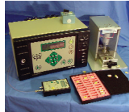
Vacuum pressure differential leak testing of a pharmaceutical liquid container.
