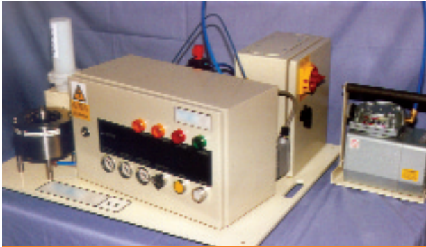
Vacuum pressure differential leak testing of a pharmaceutical liquid container.
